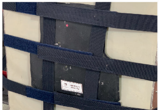
NIJ 0101.06 STANDARD TESTING: 6 SHOTS CLAY ROME #1
